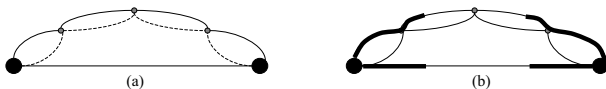
Fig. 4. The Rerstarting Primal-Dual avoids the mistake of the Naive Primal-Dual. Part (a) shows duplication of the edges. Part (b) shows the components growing along the respective edges.
